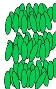
Figure 3. Arrangement of molecules in a liquid crystal.
