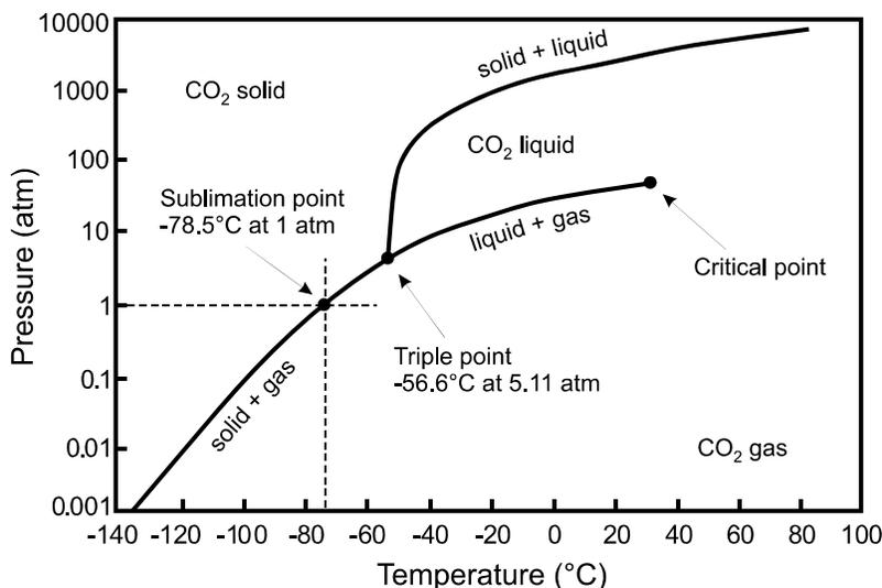
Pressure-Temperature phase diagram for  $\text{CO}_2$ .
